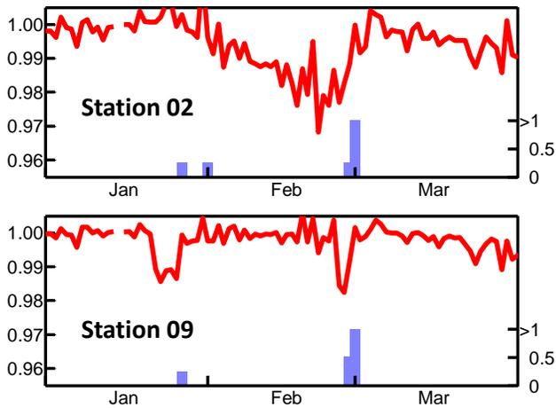
Fig. 5. Example of spatial variation in measured soiling ratio. Top and bottom graphs show soiling ratio results (left axes) from two measurement stations on east (station 02) and west (station 09) sides of power plant C. Results from each station correlated with those from nearby stations, indicating an east-west variation in soiling during January and February. Bars show rainfall in mm (right axes).
