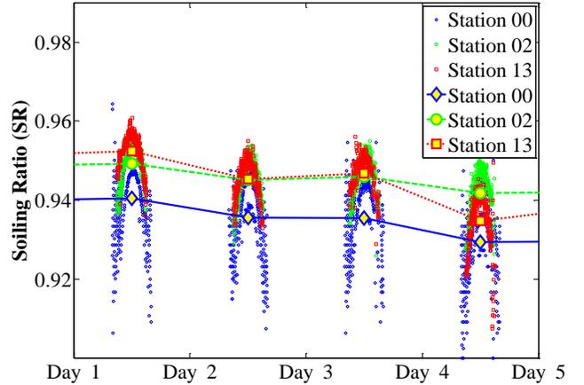
Fig. 2. Soiling ratio measurements from three measurement stations at site A over a four day period. Small symbols show instantaneous readings, taken once per minute, which vary throughout the day due as discussed in the text. Large symbols show daily averaged values.
