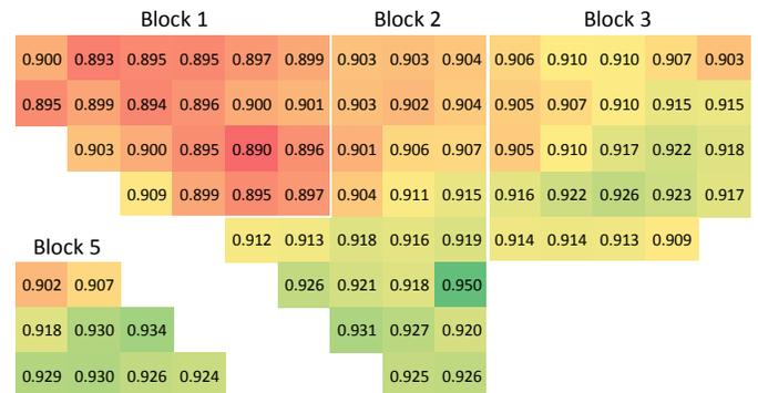
Fig. 7. Map of relative PPI at power plant D in late Oct., showing spatial variation in plant performance by inverter and confirming the trend shown by soiling measurement stations in Fig. 6.
