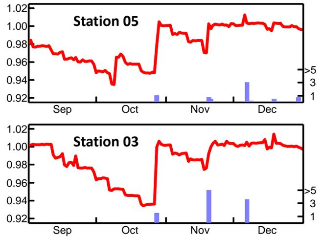
Fig. 6. Example of spatial variation in measured soiling ratio (left axes) at power plant D. Top: station 05. Bottom: station 03. Station 05 shows a recovery event in mid-October that is not apparent at Station 03. Bars show rainfall in mm (right axes).
