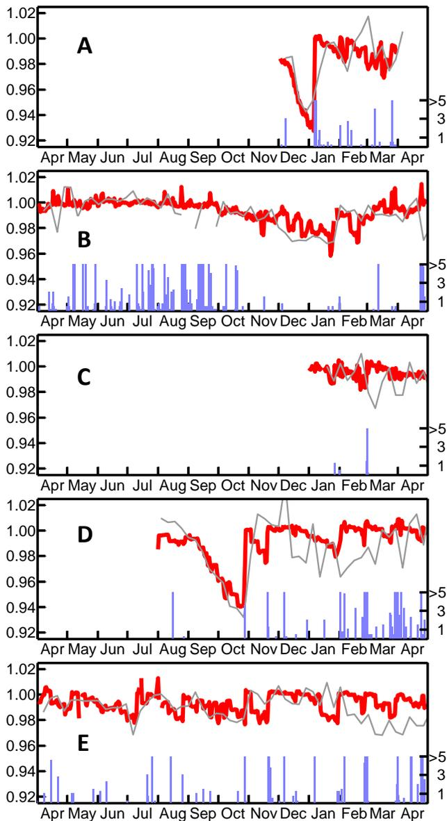
Fig. 3. Time-series plots of daily soiling ratio (thick line) and normalized weekly PPI (thin line) for the five PV power plants from April 2013 through April 2014. Bars show rainfall in mm (right axes).
