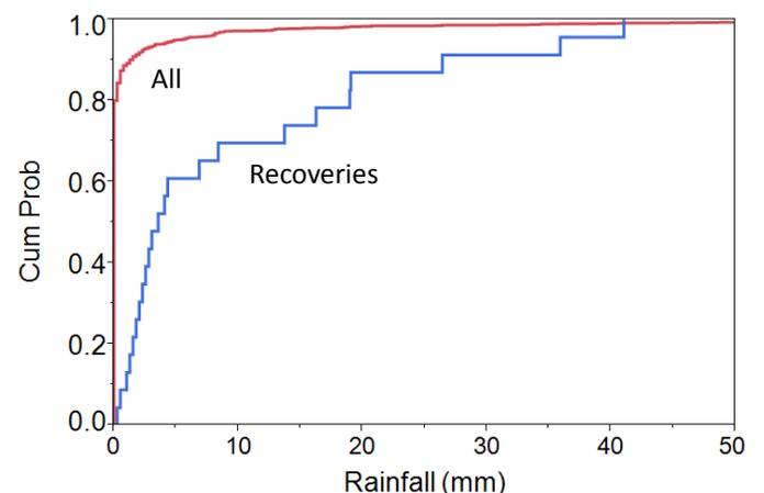
Fig. 8. Cumulative probability (left axis) of rainfall events by rainfall quantity in millimeters (bottom axis), shown for all rainfall events and for rainfall events that produced recoveries in the soiling ratio. From the recovery curve we estimate a rainfall threshold of  $\sim 3.5$  mm required to produce soiling recovery with 50% probability.
