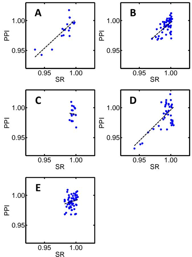
Fig. 4. Measured weekly average power plant performance ( $PPI$  axes) versus measured weekly average soiling ratio ( $SR$  axes) for the five PV power plants.
