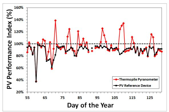
Figure 3: PV system Performance Index as calculated with pyranometer insolation data (red diamonds) and PV reference device insolation data (black circles). Note the regions where the use of the pyranometer clearly introduced error into Performance Index calculations, showing values greater than 100%.
