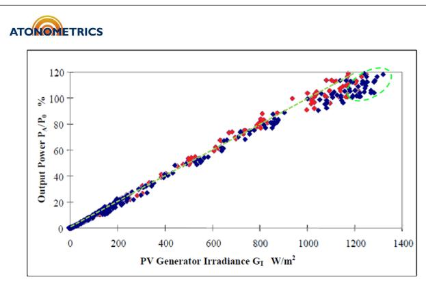
Figure 1: Hourly correlation data for the month of January, 1995, between solar irradiance as measured with a PV reference device (red diamonds) and a thermopile pyranometer (blue diamonds) from Ref. [1]. Dashed line shows a 1:1 output. The circled area highlights deviations in thermopile pyranometer data.
