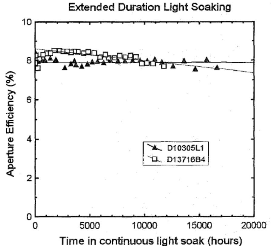
Figure 1. Performance history of two sub-modules fabricated using different recipes. The need for long term testing is apparent.
