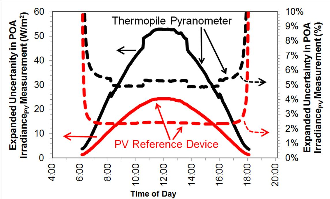
Figure 4: Typical, clear-sky expanded uncertainties in plane of array irradiance measurements made with a thermopile pyranometer and a PV reference device. The left y-axis corresponds to the solid curves and gives the uncertainties in units of  $W/m^2$ , while the right y-axis corresponds to the dashed curves and gives the uncertainties in percentages of the measured irradiance.
