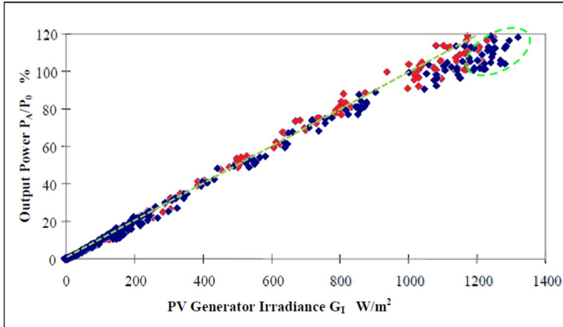
Figure 1: Hourly correlation data for the month of January, 1995, between solar irradiance as measured with a PV reference device (red diamonds) and a thermopile pyranometer (blue diamonds) from Ref. [1]. Dashed line shows a 1:1 output. The circled area highlights deviations in thermopile pyranometer data.
