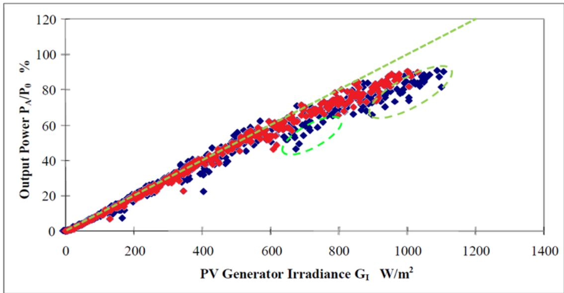
Figure 2: Hourly correlation data for the month of January, 1995, between solar irradiance as measured with a PV reference device (red diamonds) and a thermopile pyranometer (blue diamonds) from Ref. [1]. Dashed line shows a 1:1 output. The circled areas highlight deviations in thermopile pyranometer data
